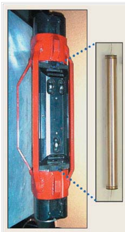
Fig. 5. A fiber optic sensor station: 3C accelerometer (right), production tubing carrier (left).
