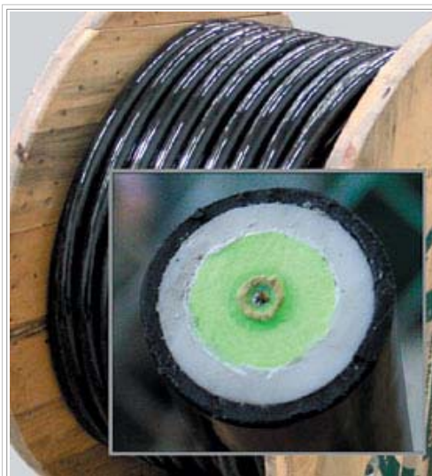
Fig. 3. For streamer applications, a special, tough urethane-based elastomeric material is applied over the core to isolate shear noise, eliminating the need for oil filling.
